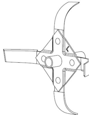
L means left blade, which is different from right blade (R).
