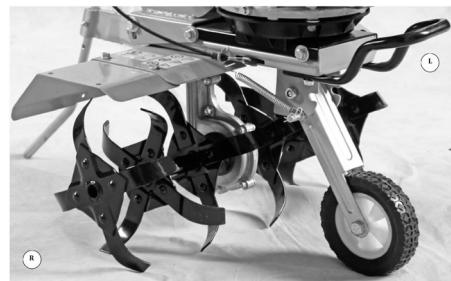
**Notes:** L means left blade, which is different from right blade (R).
